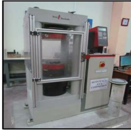
Figure 2. Toni/Technik 3.000 KN testing equipment.
